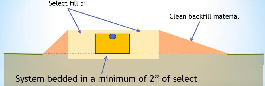
System bedded in a minimum of 2" of select fill to be considered entirely in select septic fill.
