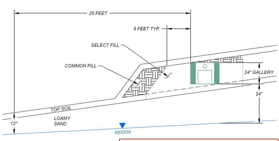
MLSS IS BASED ON RECEIVING SOIL DEPTH OF (24" + 12") / 2 = 18"
