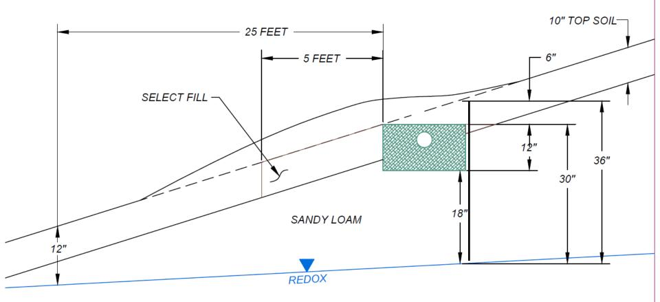
MLSS IS BASED ON RECEIVING SOIL DEPTH OF (36" + 12") / 2 = 24"
