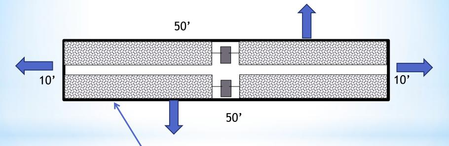
Spread can be measured around the perimeter of leaching system
