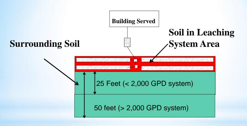
RS Depth = average depth of receiving soil in system area and surrounding soil
