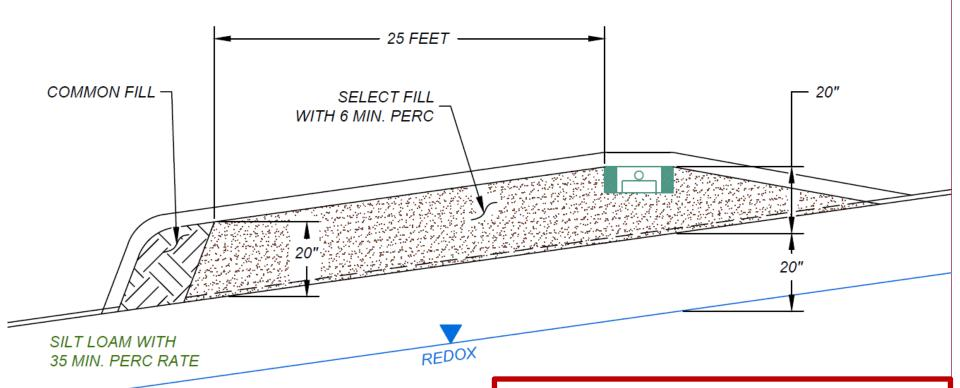
MLSS IS BASED ON RECEIVING SOIL DEPTH OF (40 + 40) / 2 = 40"
