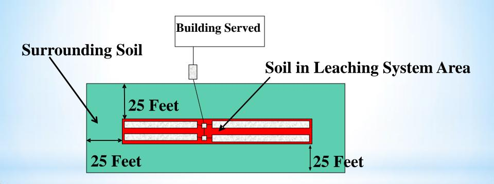
RS Depth = average depth of receiving soil in system area and surrounding soil.
