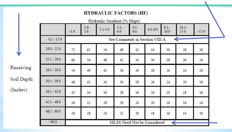
RS Depth: means the average depth of soil (soil in leaching system area and surrounding soil) measured down to the restrictive layer.
