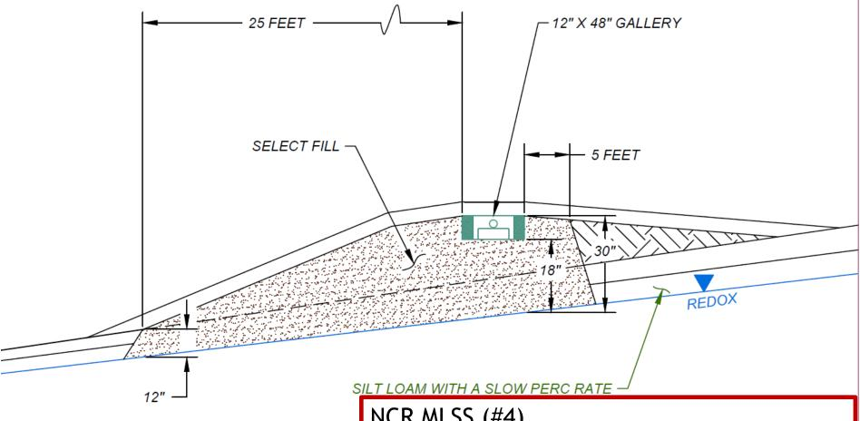
NCR MLSS IS BASED ON RECEIVING SOIL DEPTH OF (30" + 12") / 2 = 21"
