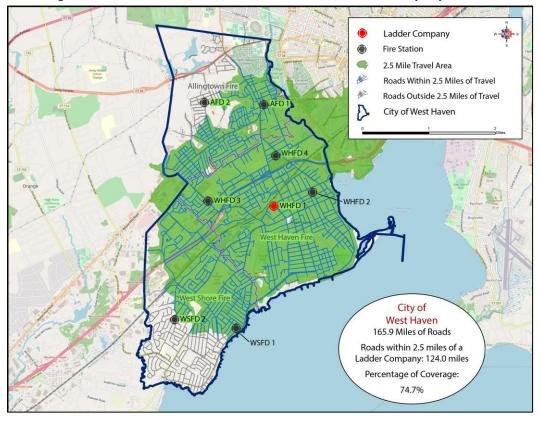
Figure 55: Fire Station Distribution, 2.5-Mile ISO Ladder Company Criteria
