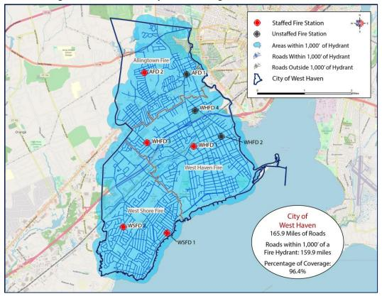
Figure 56: West Haven Hydrant Coverage, ISO 1,000-Foot Criteria
