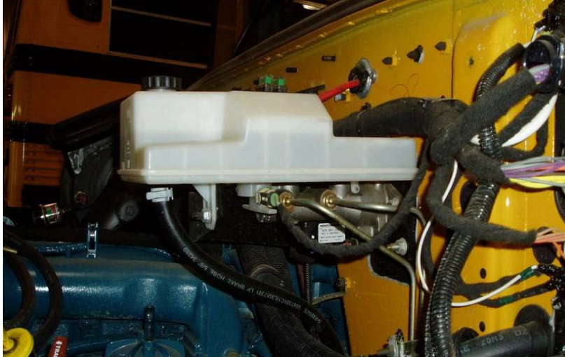
This is the firewall-mounted master cylinder.
